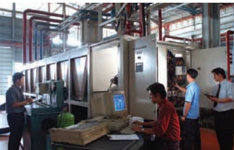
State-of-the-art ARI rated testing facility for packaged chillers at Dunham-Bush's manufacturing plant.
