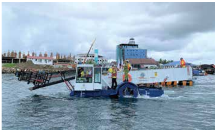
Trash Skimmer Boat deployed for seaboard cleansing of floating debris and garbage at the open sea areas.
