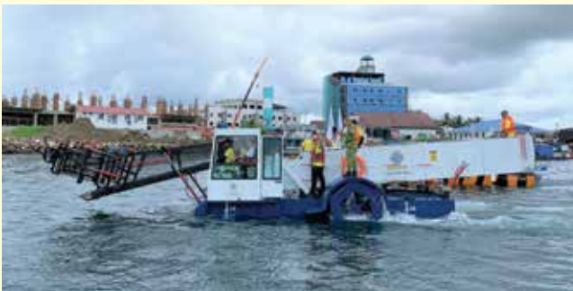
The Trash Skimmer Boat deployed for seaboard cleansing of floating debris and garbage.
