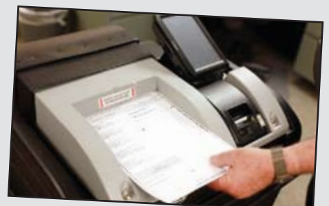
Demonstration on how a paper ballot would be inserted into the Unisyn OpenElect® vote computation and archive machine.
