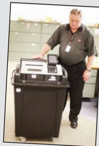
Mr. Randy Wertz, the Voter Registrar of Montgomery County in Virginia State, shows off a Unisyn OpenElect® vote computation and archive machine. The machines leave a polling paper trail, helpful if votes need to be recounted, but many polling places must cut costs to afford them.
